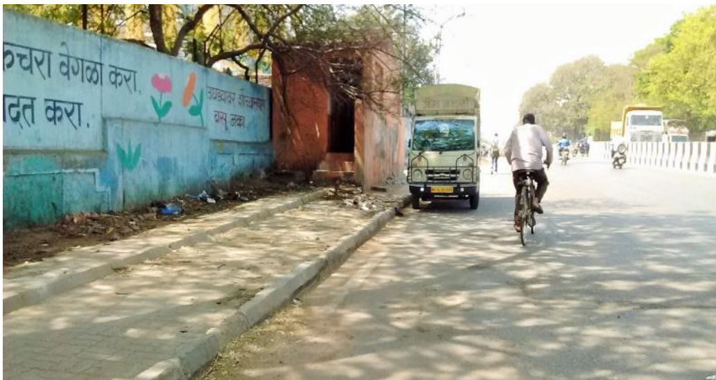
Figure 15: Cyclists being forced to use the carriage way because of unplanned services in the NMT lanes (like public toilets)
