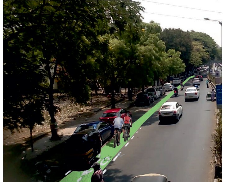
Painted cycle lane in collector roads
