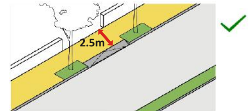
Ramp within footpath at edge only if clear walkway width available at ramp is minimum 2.5m
