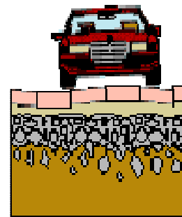
In case of clayey soil, geo-textiles help keep the overlying sub-base material from sinking into a clayey or softish sub-grade.
