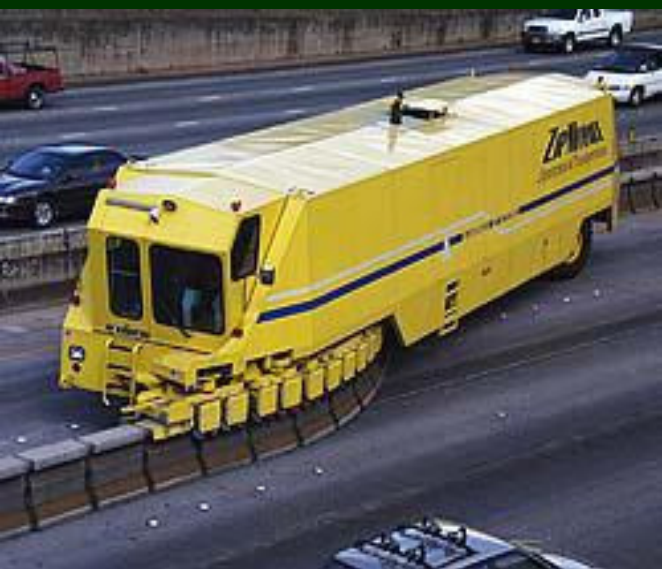
Zipper lane (movable concrete barriers) on a Hawaiian interstate freeway.
