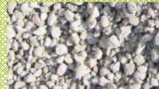
Recycled crushed concrete
