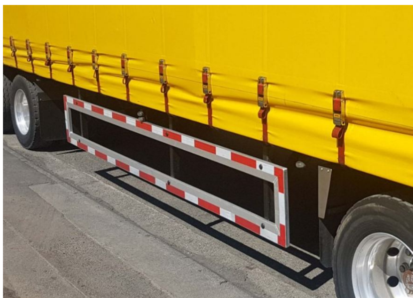
Figure A.22: Side under-run guards on truck. (Source: www.drivingtests.co.nz/resources/what-is-side-underrun-protection-on-a-truck-or-trailer/ )
