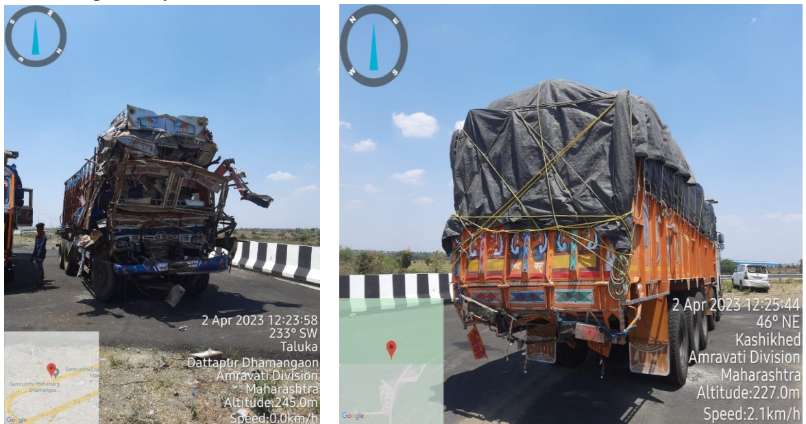
Figure 32: Accident caused due to head-tail collision with breakdown vehicle.
